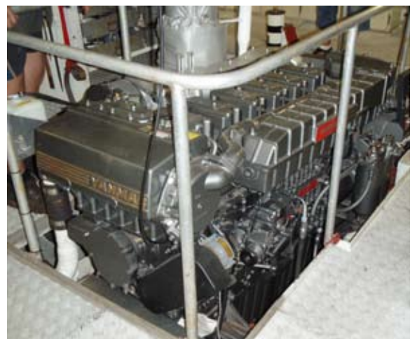
One of two Yanmar 6AY engines installed
